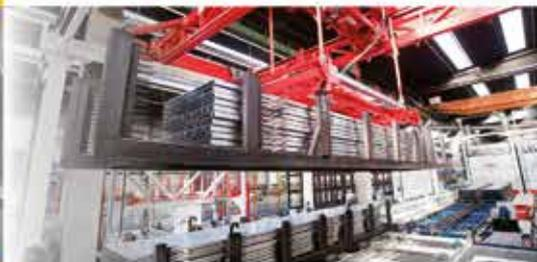
Fully automatic systems for extrusion plants to handle flows of material, from the ageing oven to the storage area, including Stacker/De-Stacker, Basket Handling Systems, Packing Lines and Automatic Storage Systems with the newly-born company named WeStore.
